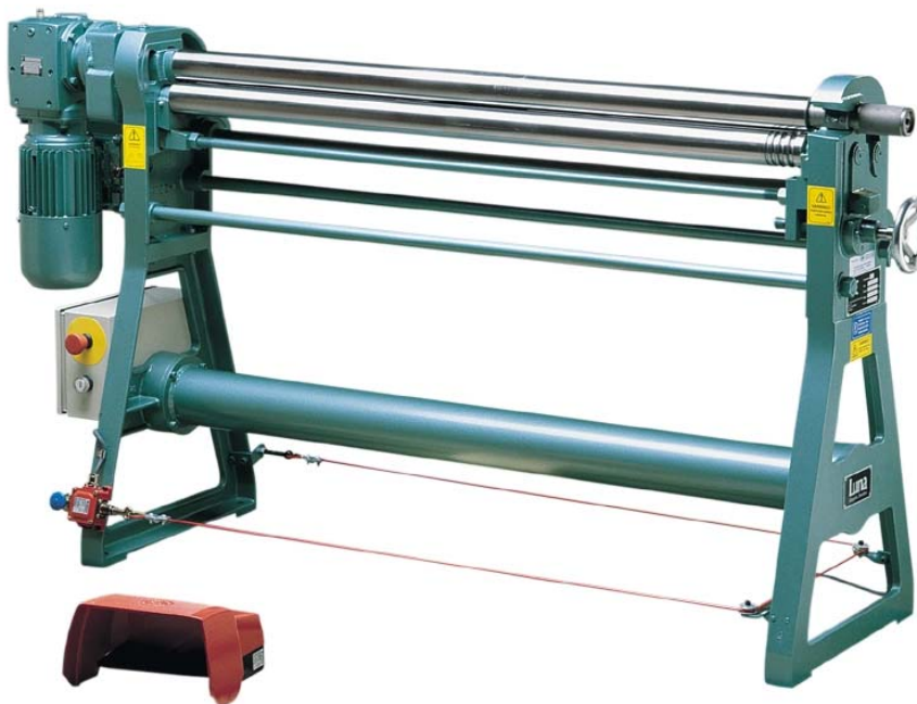
The Titan 4135 Series machine with roll diameter of 2.36"
